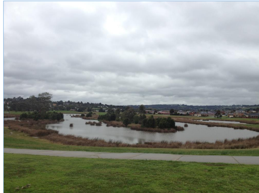
Wetland for pretreatment of water used in Troup Creek stormwater recycling facilities (Melbourne)
